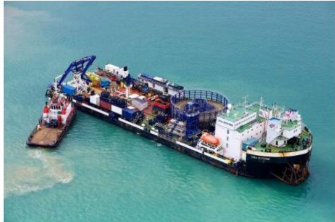
A boat like this would be used to lay the subsea electricity cables from a power plant near Le Havre to a landing point in Eastney, Portsmouth.
